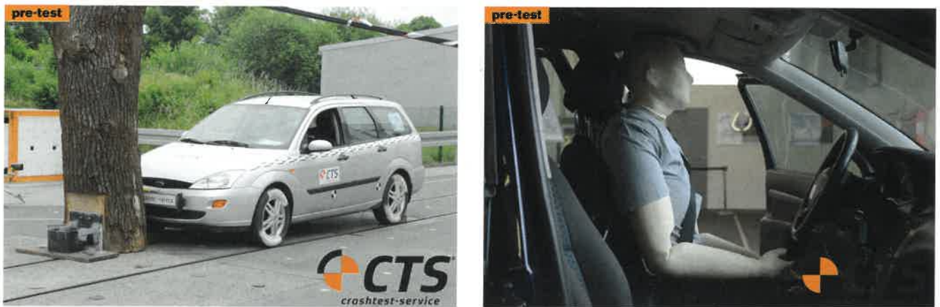
Figure 2: Collision configuration for the series of tests with a head-on collision with a tree accounting for 40% coverage of the vehicle (left) and the PRIMUS dummy used for the tests, positioned in the vehicle (right)
