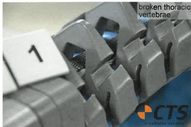
Figure 20: Injuries to the unbelted PRIMUS dummy
