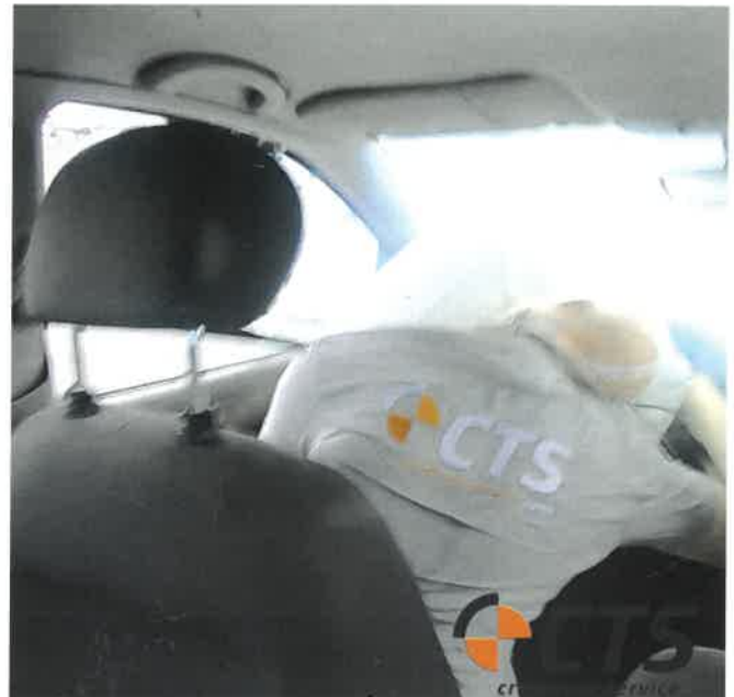
Figure 15: Significant rotation of the head when immersing in the airbag (properly belted)
