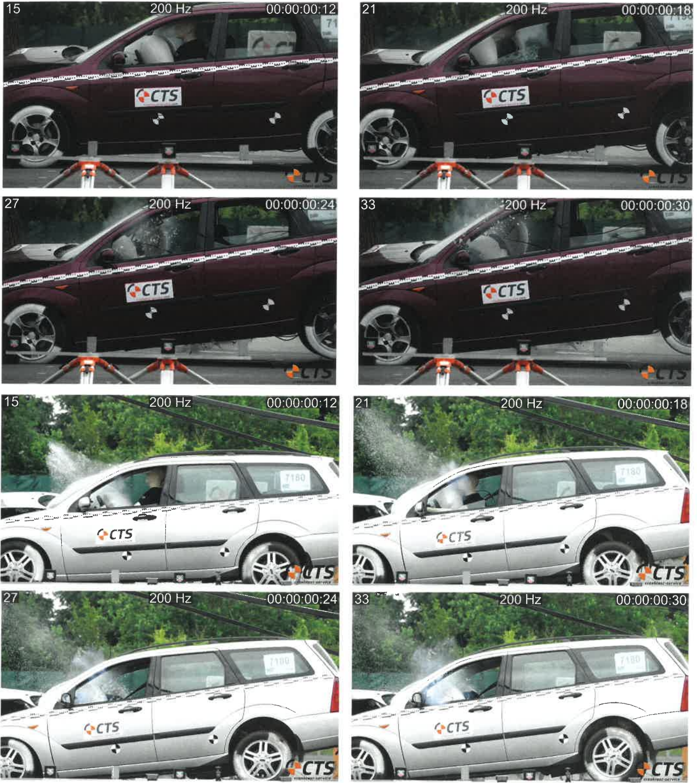
Figure 4: Motion sequence for unbelted (top), poorly belted (bottom) and properly belted PRIMUS (next page)
