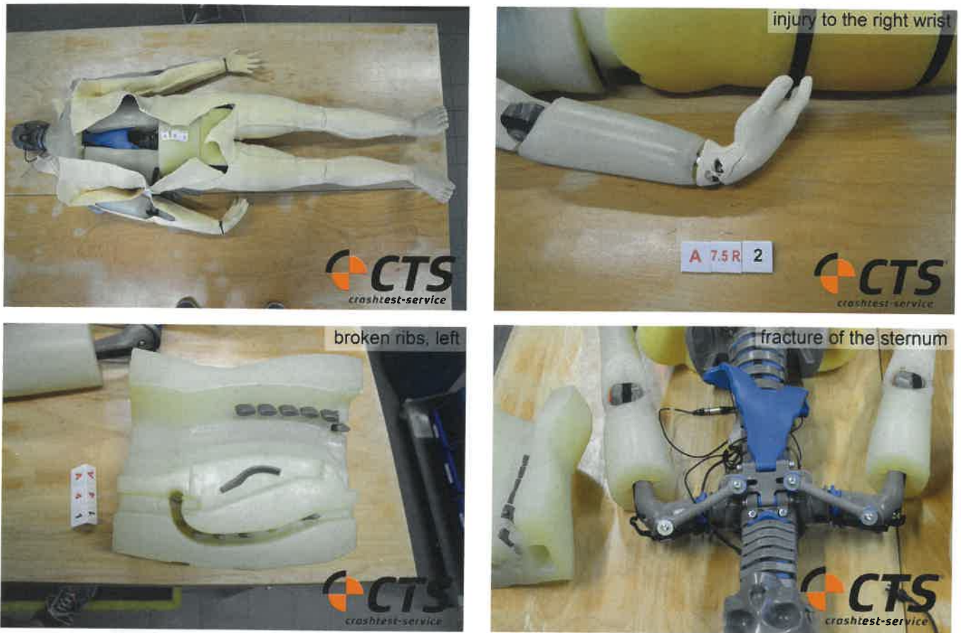
Figure 22: Injuries to the properly belted PRIMUS dummy
