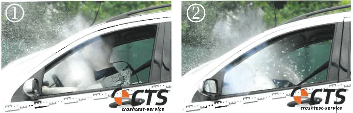
Figure 11: Impact of the poorly belted occupant with the airbag (1) and the steering wheel (2)
