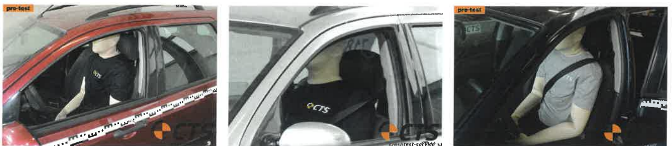
Figure 3: Degree of seat belt use for the tests: not wearing a seat belt (left), the chest strap worn under the left shoulder (middle), and the seat belt worn correctly (right)
