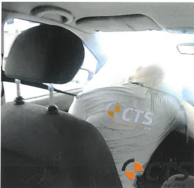
Figure 15: Significant rotation of the head when immersing in the airbag (properly belted)
