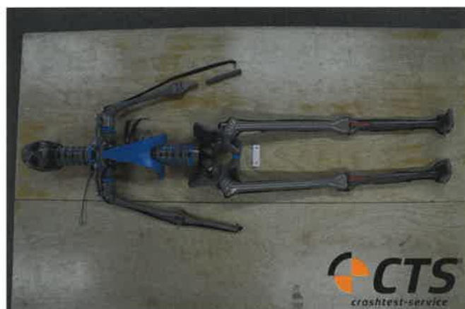
Figure 20: Injuries to the unbelted PRIMUS dummy
