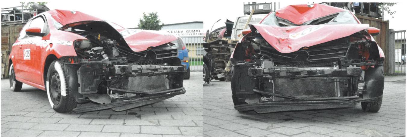
Figure 5: Damage of the VW Polo after dismantling the bumper cover
