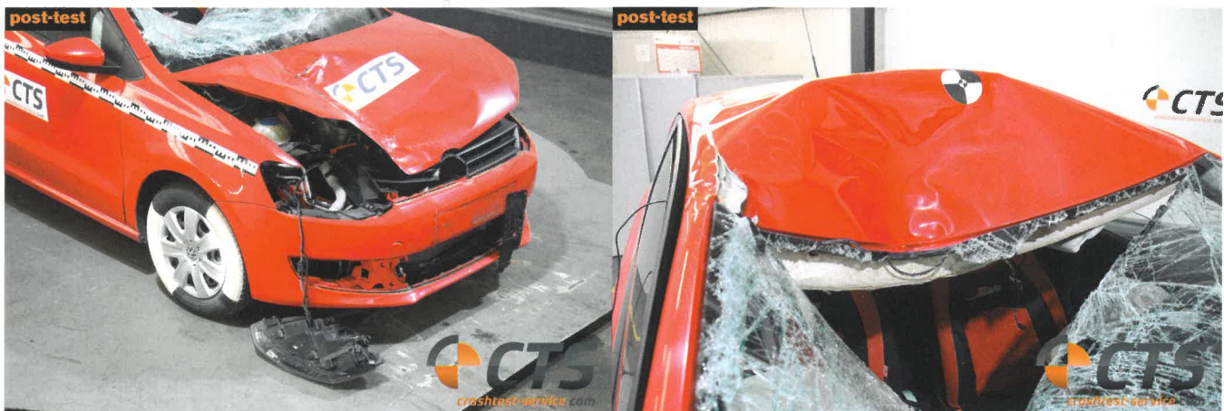
Figure 4: Hood and roof damage on the VW Polo at v = 109 kph.
