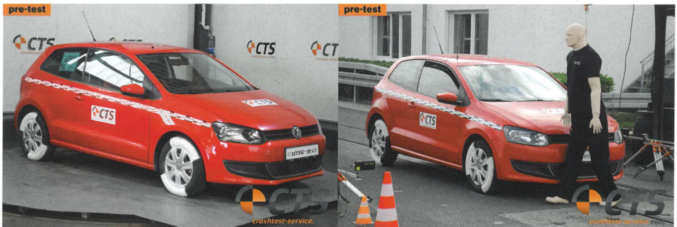
Figure 1: Crash vehicle VW Polo 6R (left) and impact situation with Biofidel dummy (right) for the high-speed test with v = 109 kph
