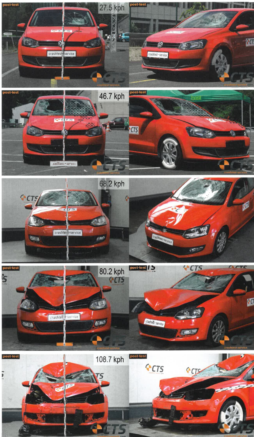
Figure 7: Change in the damage pattern (impact against Bio-fidel) on the VW Polo 6R with increasing speed from 27.5 to 108.7 kph in the front and side view
