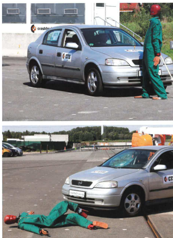
Fig.3 CTS crash test at 32 kph impact and final position
