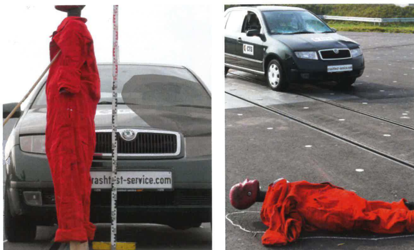
Fig.2 CTS crash test at 37 kph impact and final position
