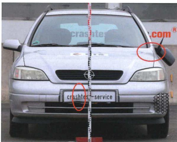
Fig.5 CTS crash test: comparison of the dent offset between Figures 3 and 4
