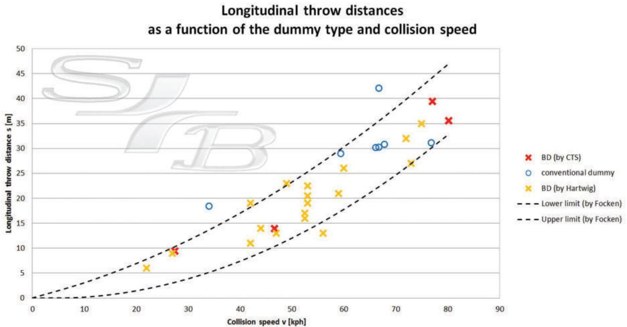
Figure 11: Graph with throw distances of the different dummy types as a function of the collision velocity – trend line according to Focken<sup>6</sup>
