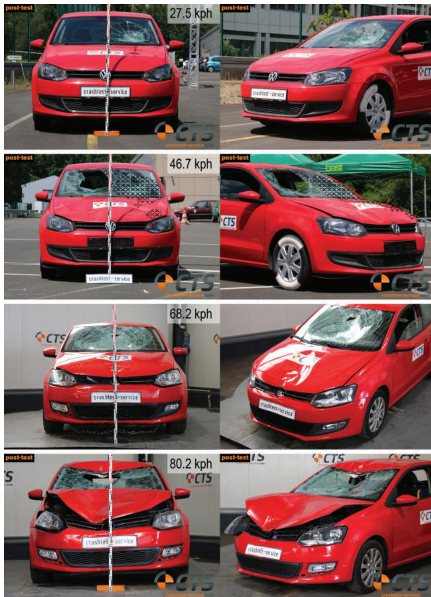
*Figure 3: Frontal and side view of the change in the damage pattern (impact with biofidelic dummy) on the VW Polo 6R with increasing collision velocity from 27.5 to 80.2 kph*
