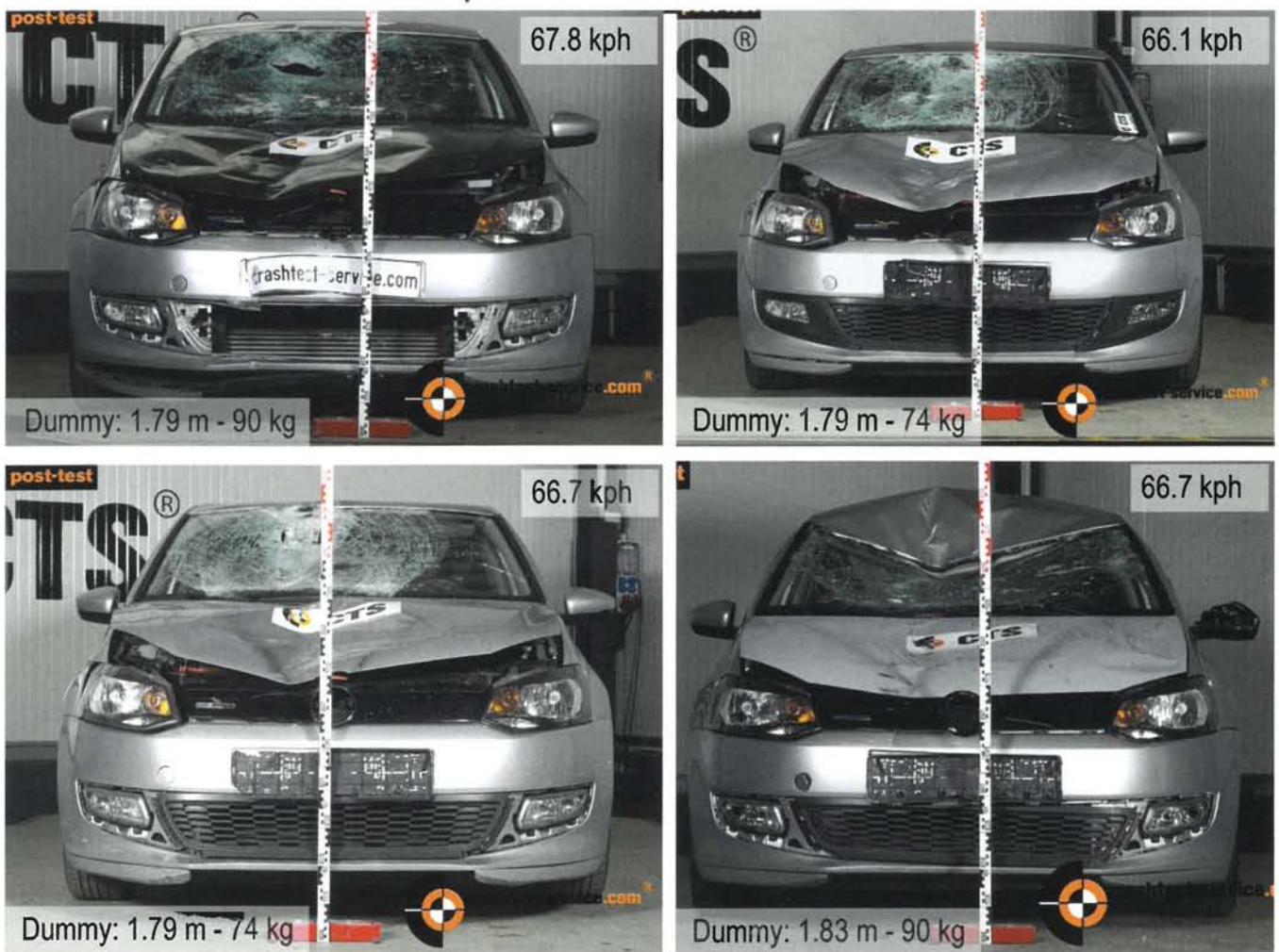
Figure 9: Comparison of the damage to the VW Polo 6R after an impact with a conventional dummy in the velocity range from 66 to 68 kph
