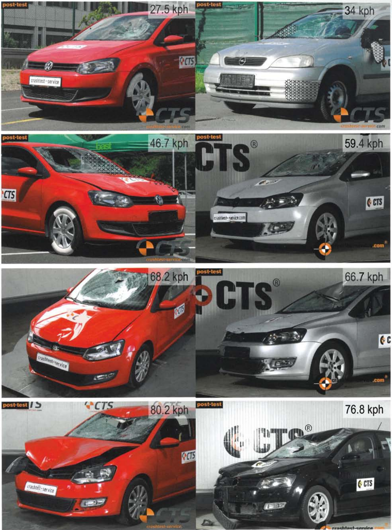
Figure 6: Comparison of the damage to the VW Polo 6R after an impact with the biofidelic dummy (left) and a conventional dummy (right) with increasing collision velocity (side view)
