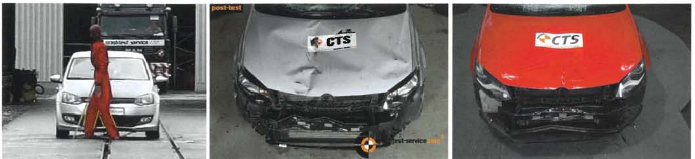
Figure 8: Step position for the impact with the conventional dummy (left) and the resulting cross-member deformation (centre) at v = 70 kph; comparison of the frontal damage after an impact with the biofidelic dummy (right)
