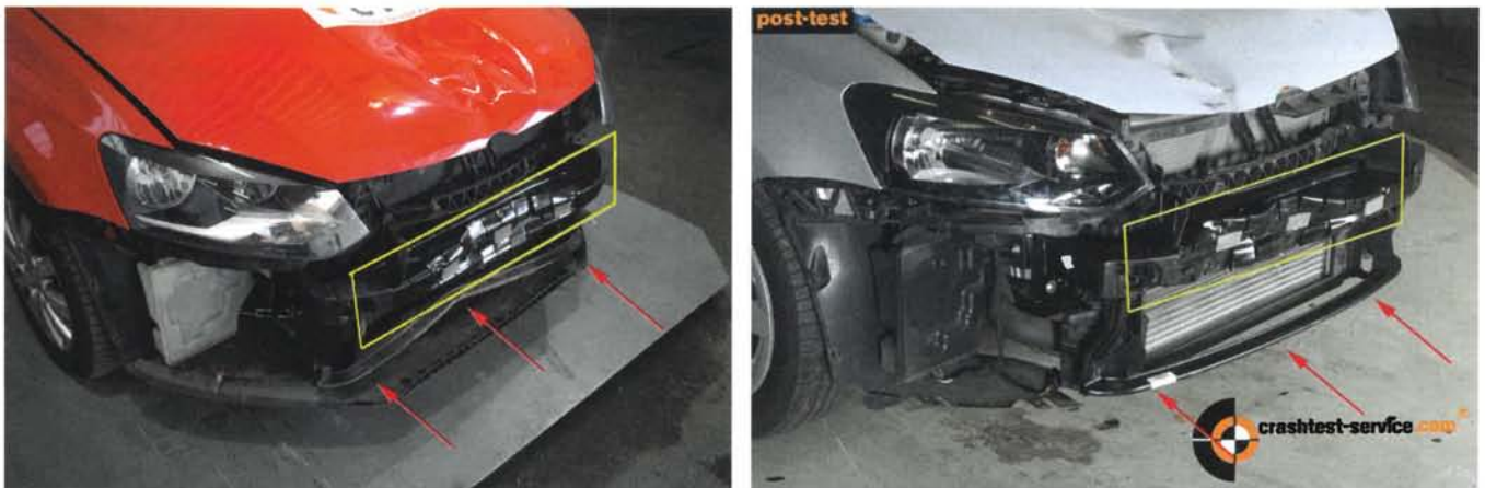
Figure 7: Comparison of the frontal damage to the crash vehicle (bumper removed) after a collision with the biofidelic dummy (left) and a conventional dummy (right) at v = 70 kph
