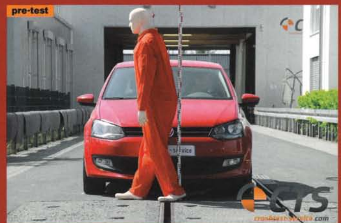
Figure 1: Crash test vehicle VW Polo 6R (left) and impact situation with a biofidelic dummy (right) for the crash series performed
