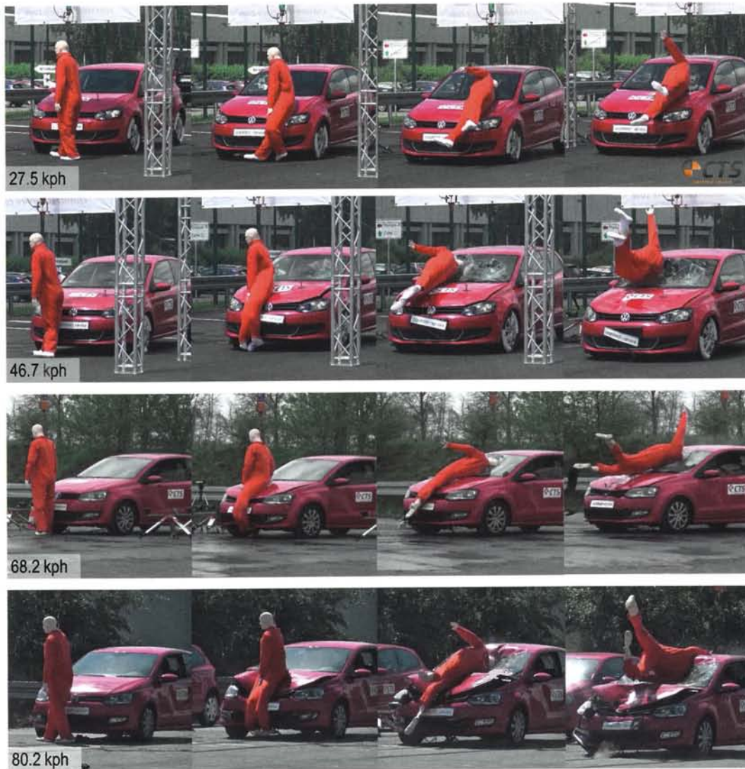
Figure 4: Motion sequence of the biofidelic dummy and head impact height with increasing collision velocity
