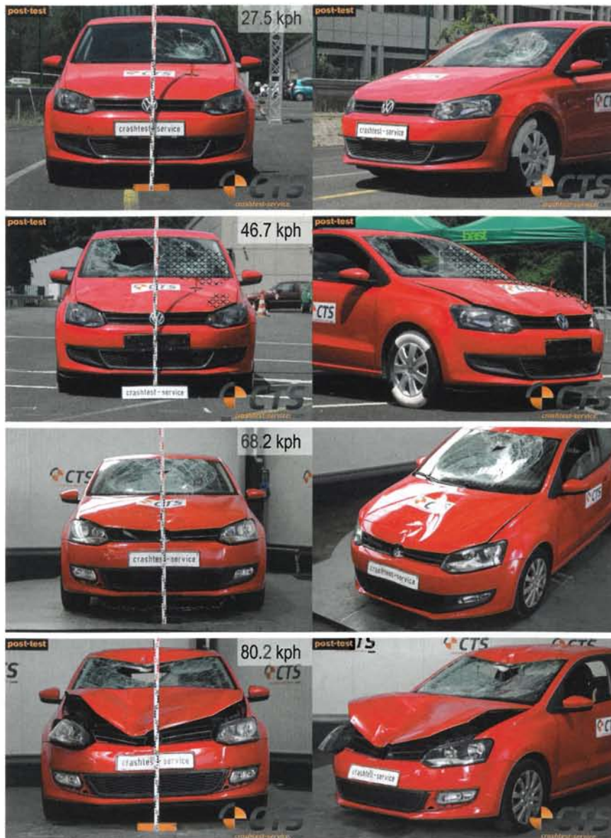
Figure 3: Frontal and side view of the change in the damage pattern (impact with biofidelic dummy) on the VW Polo 6R with increasing collision velocity from 27.5 to 80.2 kph
