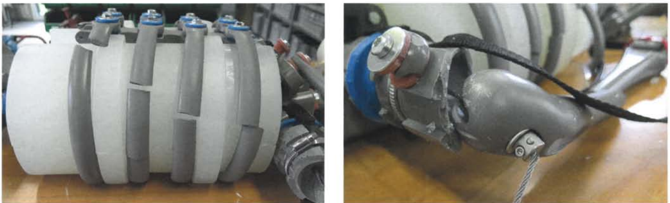
Figure 12: Biofidelic dummy with serial rib fracture and shoulder joint injuries at a collision velocity of approx. 70 kph
