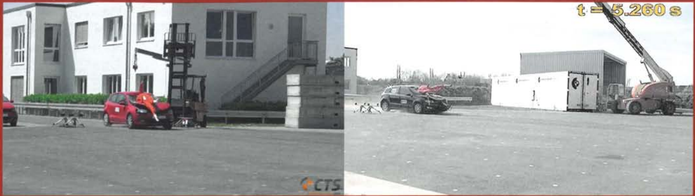
Figure 2: Re-enactment (left – biofidelic) of the already available crash tests (right – conventional) – collision velocity here: v = 68 kph
