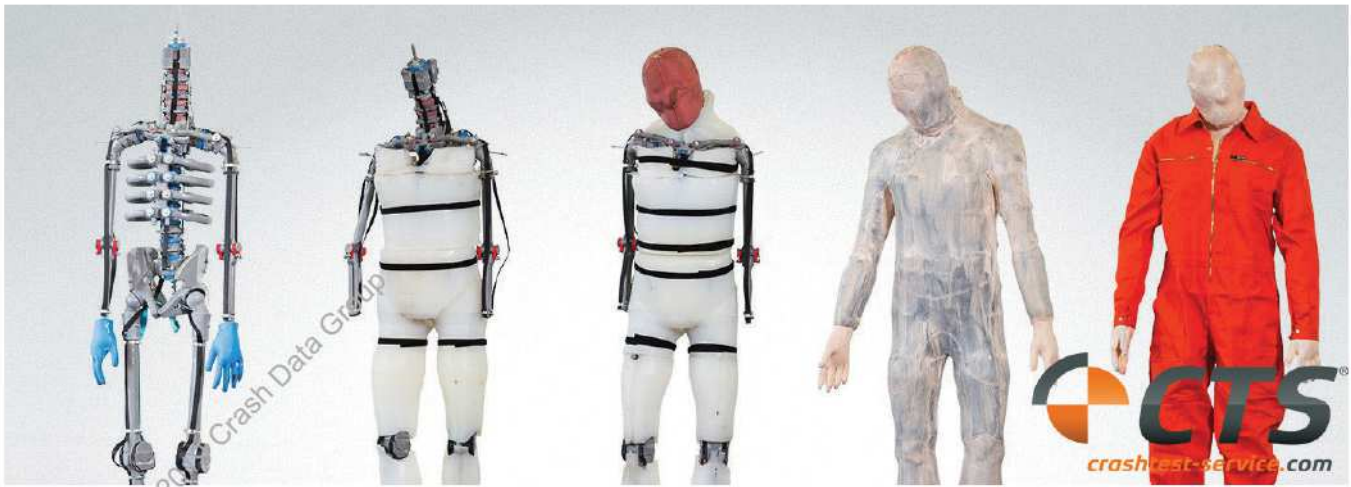
Figure 2: Each stage of the biofidelic dummy production process
