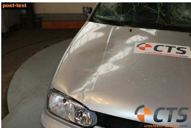
Figure 8: Damages caused to the bonnet
