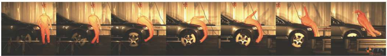
Figure 11: Movement sequences during the test with the biofidelic dummy
