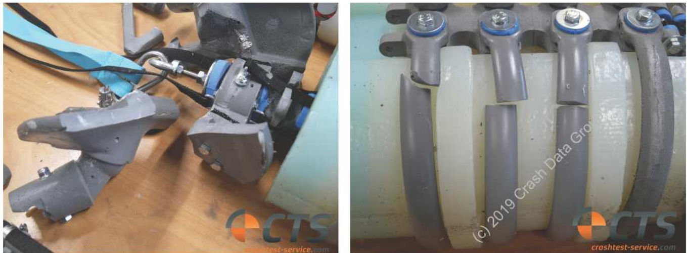
Figure 25: An autopsy of the biofidelic dummy after a collision
