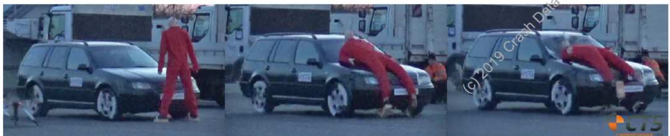
Figure 19: The movement sequence of the biofidelic dummy in a head-on crash impact configurations
