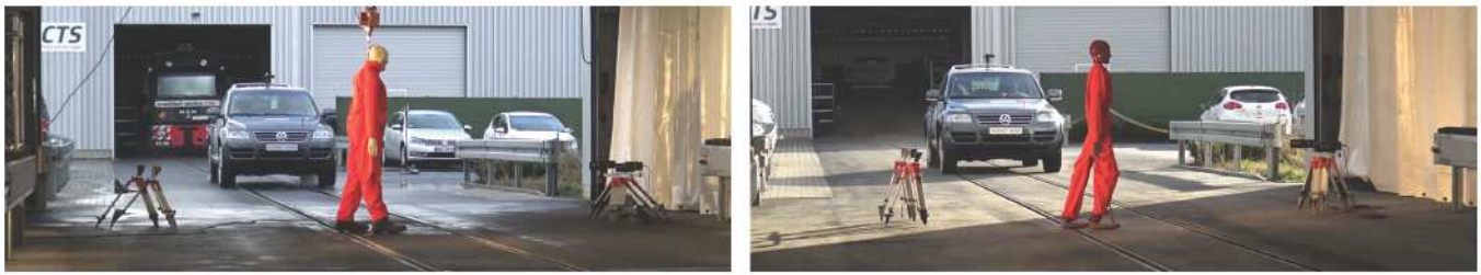
Figure 9: The test setup, where a biofidelic and a NAMI-dummy under identical conditions are impacted with a VW Touareg
