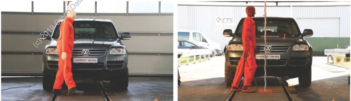
Figure 10: The test setup, where a biofidelic and a NAMI-dummy under identical conditions are impacted with a VW Touareg
