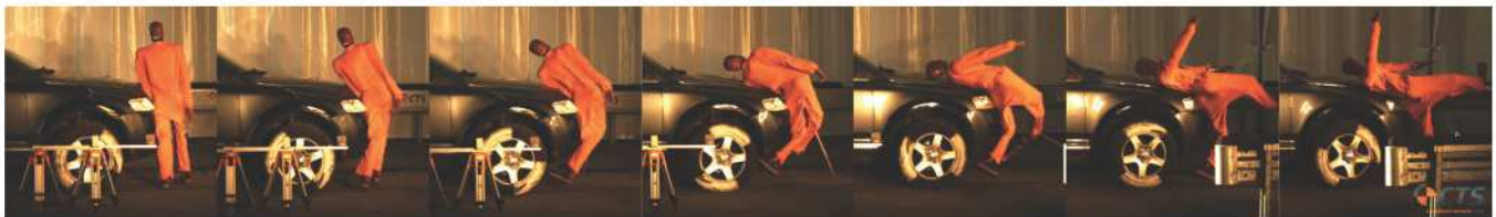
Figure 12: Movement sequences during the test with the NAMI-dummy
