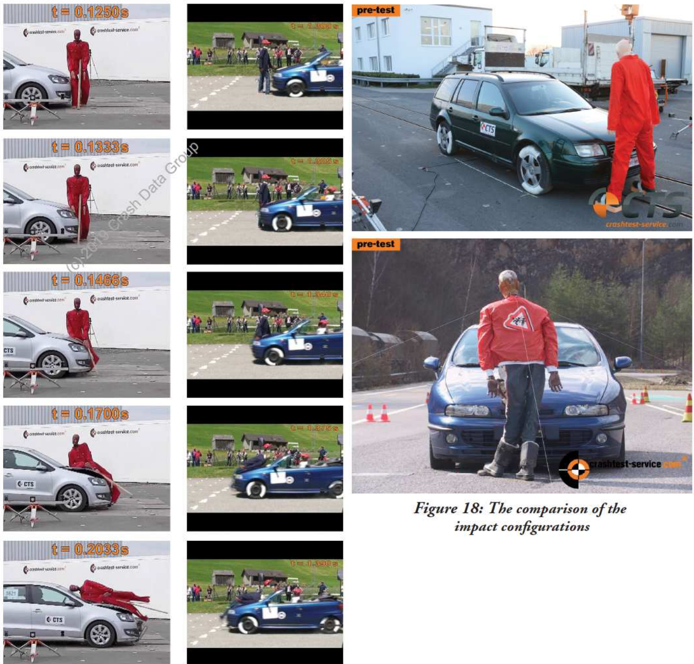
Figure 17: Carrying-characteristic of the pedestrian
