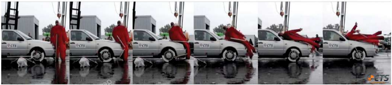
Figure 4: The movement sequences of the conventional dummy
