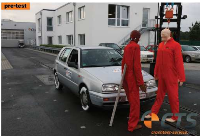
Figure 3: The impact configuration with a conventional (NAMI-) dummy in vehicle plan view on the left side
