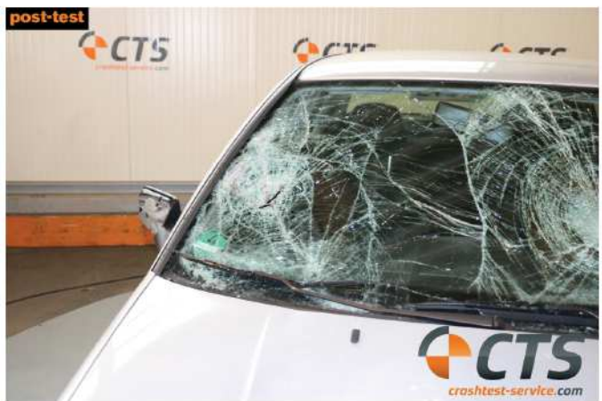
Figure 7: Fracture pattern in the windscreen
