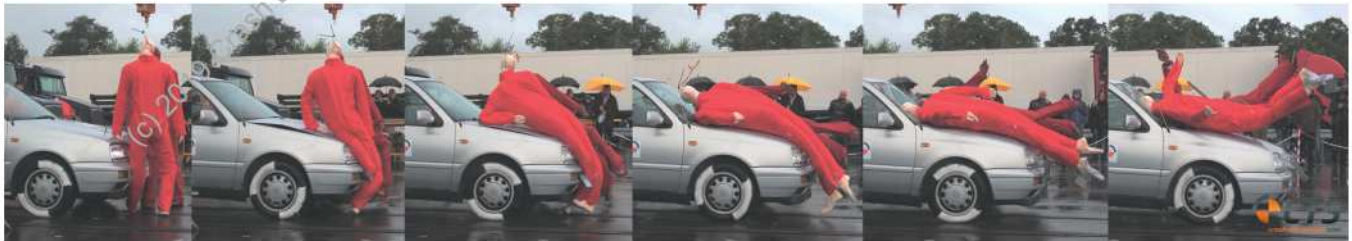
Figure 5: The movement sequences of the biofidelic dummy impacted by a passenger car (mirrored)
