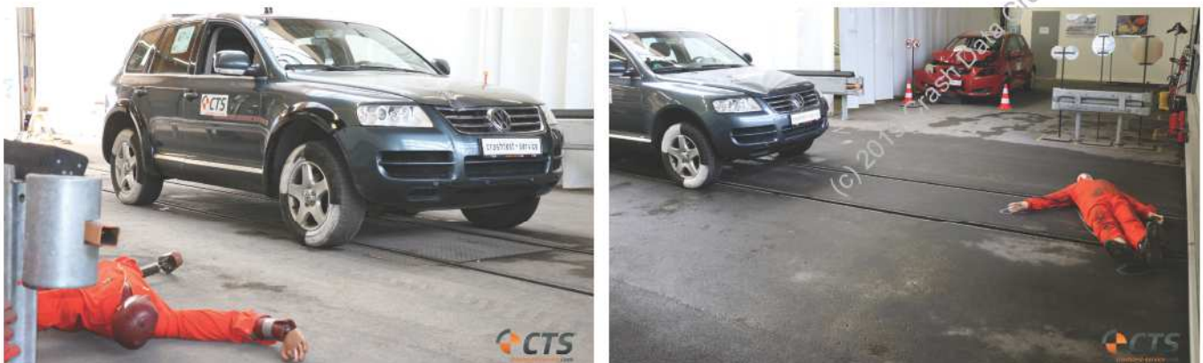
Figure 13: End positions of the different dummy types
