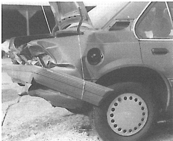
FIG. 4. Moderate deformation in FS 90.
