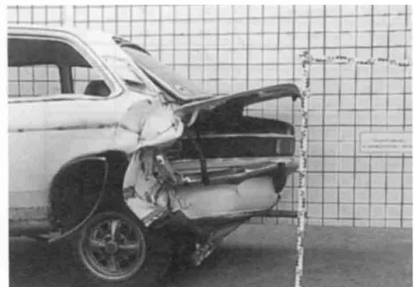
Versuch 10: v_k = 51 \text{ km/h} , a_{\text{gemittelt, KADETT}} = 3,6 \text{ g} , v'_{\text{KADETT}} = 29 \text{ km/h} , \Delta v' = 3 \text{ km/h}
