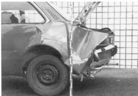
Versuch 10: v_k = 51 \text{ km/h} , a_{\text{gemittelt, KADETT}} = 3,6 \text{ g} , v'_{\text{KADETT}} = 29 \text{ km/h} , \Delta v' = 3 \text{ km/h}
