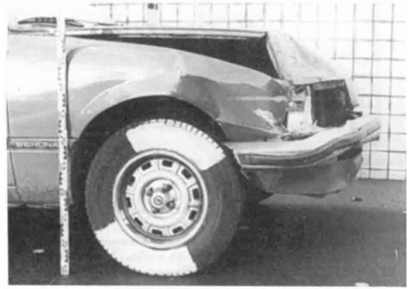
Versuch 11: v_k = 32 \text{ km/h} , a_{\text{gemittelt, KADETT}} = 2,8 \text{ g} , v'_{\text{KADETT}} = 21 \text{ km/h} , \Delta v' = 3 \text{ km/h}
