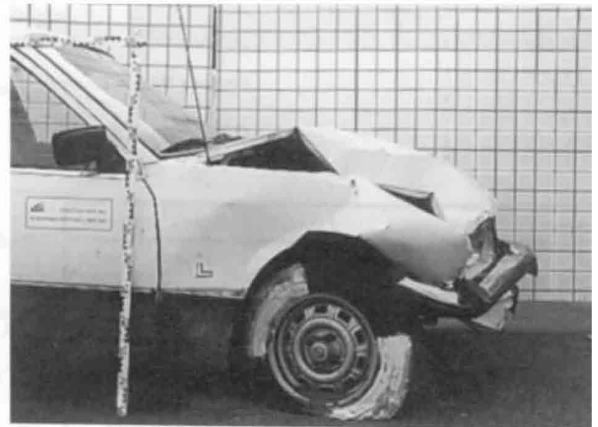
Versuch 12: v_k = 32 \text{ km/h} , a_{\text{gemittelt, KADETT}} = 2,4 \text{ g} , v'_{\text{KADETT}} = 19 \text{ km/h} , \Delta v' = 1 \text{ km/h}
