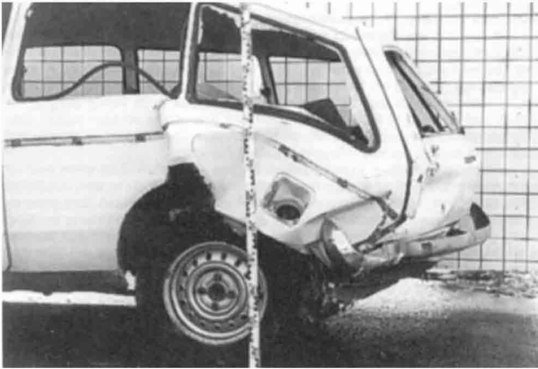
Versuch 11: v_k = 32 \text{ km/h} , a_{\text{gemittelt, KADETT}} = 2,8 \text{ g} , v'_{\text{KADETT}} = 21 \text{ km/h} , \Delta v' = 3 \text{ km/h}
