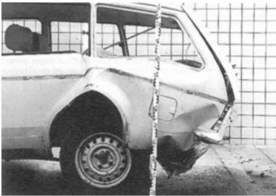
Versuch 9: v_k = 55 \text{ km/h} , a_{\text{gemittelt, KADETT}} = 4,0 \text{ g} , v'_{\text{KADETT}} = 35 \text{ km/h} , \Delta v' = 4 \text{ km/h}
