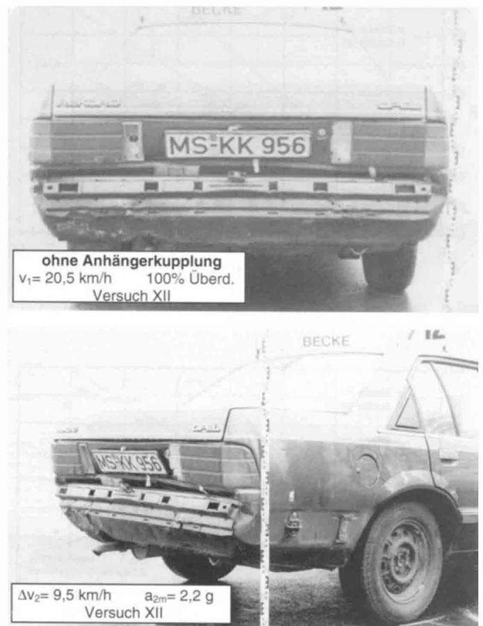
Fig. 14 Vehicle damages with or without trailer coupling
